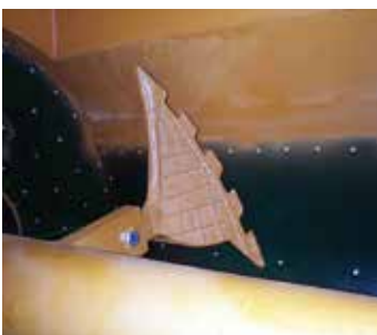
Special anti-wear mixing tool coating
